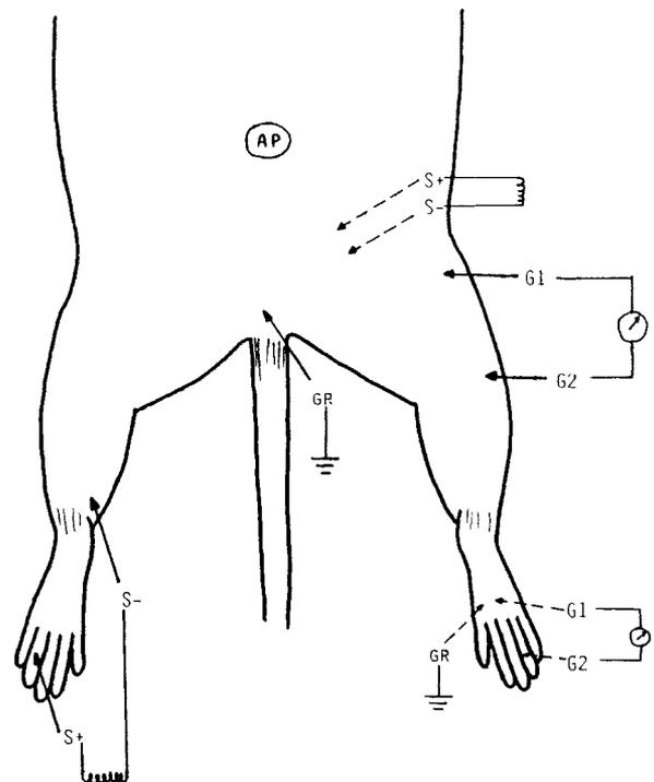
**FIGURE 1.** Schematic drawing of the electrodes placed in the rat hindlimbs for simultaneous recording of the H wave (interrupted arrows) and the extensor reflex (full arrows).
