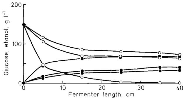
**Fig. 7.** Continuous fermentation profiles at 35°C.  $S_0 = 150 \text{ g l}^{-1}$  and increasing flow rates ( $\text{ml h}^{-1}$ ): (1) 30, (2) 65, (3) 110. ○, glucose concentration,  $\text{g l}^{-1}$ ; ● ethanol concentration,  $\text{g l}^{-1}$
