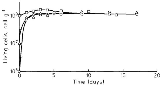
**Fig. 1.** Cell growth during fermentation inside the gel beads for various initial cell loadings (in number of living cells  $\text{g}^{-1}$  of gel):  $\square$ ,  $10^9$ ;  $\Delta$ ,  $10^7$ ;  $\circ$ ,  $10^5$
