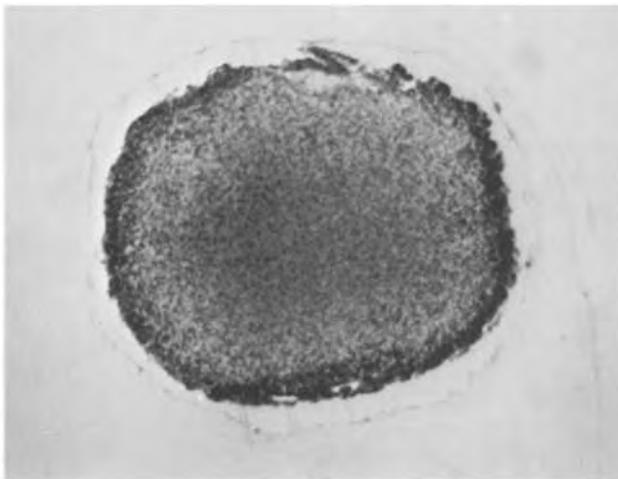
**Fig. 8.** Transversal section of a gel bead of the bottom fraction of the fermenter after a continuous experiment
