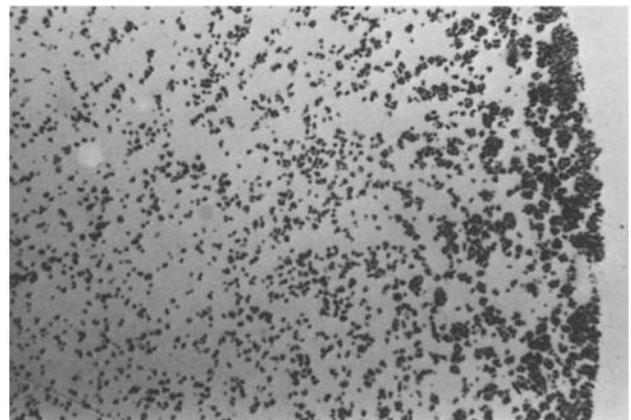
**Fig. 3.** Detail of a transversal section of a gel bead after one day fermentation (initial cell loading as in Fig. 2)
