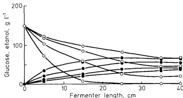
**Fig. 6.** Continuous fermentation profiles at 30°C. S<sub>0</sub>=150 g l<sup>-1</sup> and increasing flow rates (ml h<sup>-1</sup>): (1) 30, (2) 65, (3) 110, (4) 157. ○, glucose concentration, g l<sup>-1</sup>; ●, ethanol concentration, g l<sup>-1</sup>
