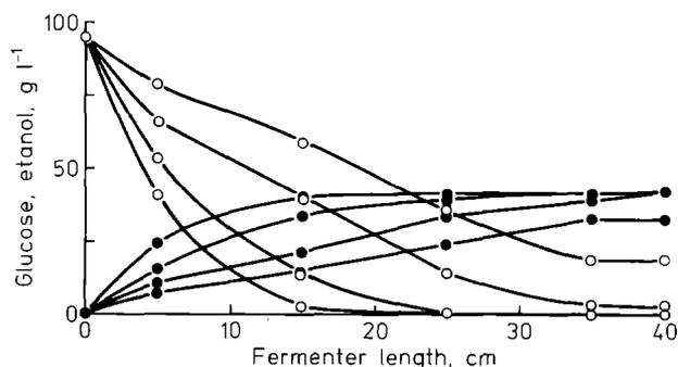
**Fig. 5.** Continuous fermentation profiles at 30°C. S<sub>0</sub>=95 g l<sup>-1</sup> and increasing flow rates (ml h<sup>-1</sup>): (1) 30, (2), 65, (3) 110, (4) 157. ○, glucose concentration, g l<sup>-1</sup>; ●, ethanol concentration, g l<sup>-1</sup>
