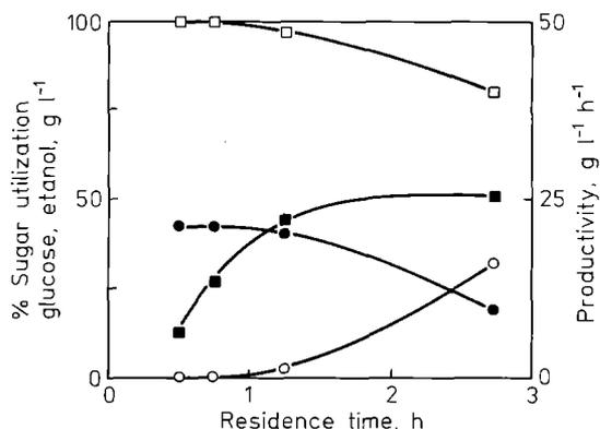
**Fig. 4.** Continuous fermentation results at various residence times for a 95 g l<sup>-1</sup> glucose feed concentration and 30°C, ● ethanol concentration in the effluent, g l<sup>-1</sup>; ○, glucose concentration in the effluent, g l<sup>-1</sup>; □, percentage of sugar utilization; ■, ethanol productivity, g l<sup>-1</sup> h<sup>-1</sup>. Residence time is calculated on liquid volume basis and productivity on total volume fermenter basis
